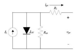
Fig. 2. Equivalent circuit diagram of PV cell
